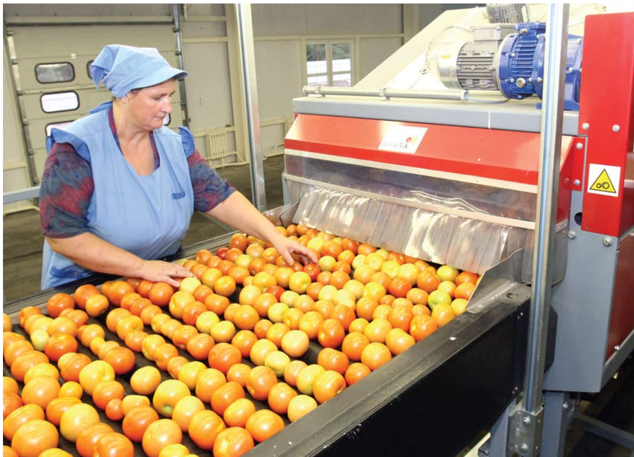
The Rudakovo greenhouse complex, Vitebsk District, has launched Belarus' first tomato sorting line with the capacity of 10 tonnes per hour. The line can sort vegetables by color and size. Trading outlets of Belarus and Russia have already expressed interest in Rudakovo tomatoes
