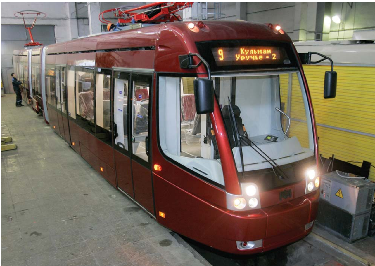
A new high-speed tram 84300M is assembled at Belkommunmash. The tram can accelerate to 120km/h and can be used for commuting
